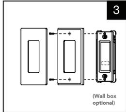
Use any Decora compatible wall plate (sold separately). Screw the wall plate base on with the trim screws provided with the wall plate.
