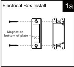
Screw the wall plate adapter to the wallbox with the provided screws. Be sure the magnet is on the bottom.
