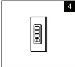
Snap the wall plate cover on and attach the xPRESS Audio Keypad. The keypad magnetically attaches to the wall plate adapter and can be removed at any time.
