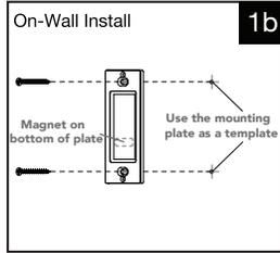
Mark the holes using the wall plate adapter and use the screws provided to screw the wall plate adapter to the wall. No other anchors are required.
