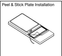
Peel plastic to reveal the adhesive strip. Stick onto a wall or furniture. The keypad magnetically attaches to the wall plate adapter and can be removed at any time.
