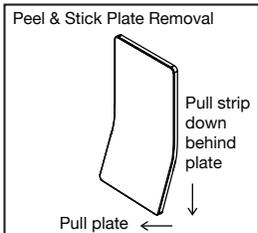
To remove the peel and stick plate, pry up the bottom and pull/stretch the adhesive strip downward.
