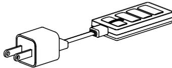
To charge, connect the USB A connector on the supplied USB cable to any 5v USB power adapter like a smart phone charger. Connect the micro-USB end to your Keypad. Charging can take up to 3 hours. When the red LED on the Keypad turns green, charging is complete.
