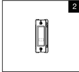
Be sure the wall plate adapter is level and tightened.
