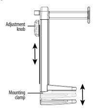
**3** Rotate the hanger up to 360° to adjust its position.
