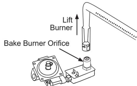
1. Remove oven racks, door and oven bottom. Remove the 1/4" hex screws securing the bake burner.
