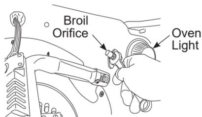
1. Remove the 1/4" hex screw securing the broil burner and allow it to hang down free of the broil orifice.
