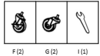
**Use the provided CASTER WRENCH (I) to tighten the CASTERS (F+G) completely. Failure to do as instructed could result in the caster stem breaking.**
