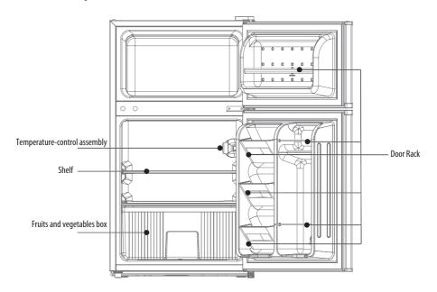
**Note:** To remove a refrigerator shelf, lift it up, then slide it out.
