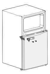
7. Place freezer chamber door on middle hinge then ÿx the top hinge,top hinge cover on left side and insert hole caps on right side.
