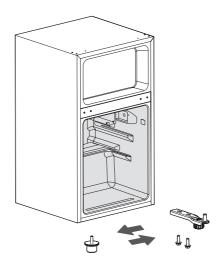
**6.** Place refrigerating chamber door on bottom hinge then fix the middle hinge on left side and insert the hole caps on right side;
