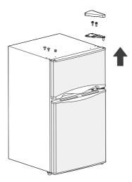
3. Remove freezer chamber door as well as middle hinge and hole cap of the other side;
