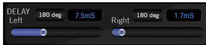
1. The delay of each input channel can be adjusted with these sliders and the numeric display.
