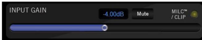
1. The input gain control is a slider that can be adjusted with the mouse, arrow keys, or by numerically entering the level in dB. The slider will move in 1 dB increments with left and right arrow key strokes. This includes any typed-in a value, such as “-2.3” dB, then an arrow key left will be “-3.3” dB.
