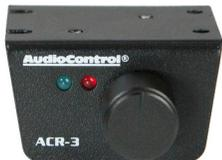
The optional AudioControl ACR-3 dash control is a dual-function remote for your DM-608/DM-810. It may be mounted under the dash using its own bracket, or through a custom hole in the dash. The endless knob should be within reach of the driver, and in a spot where the two LEDs are plainly visible. Disconnect the vehicle battery +12V and Ground connections before installation.
