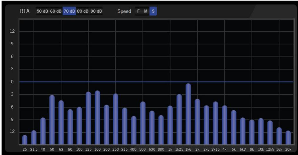
1. The input RTA shows the level of signal at the input of the DSP, post gain control (that is, after the gain control has done its thing).
