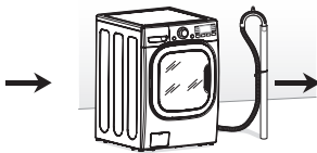
Connecting the drain line
