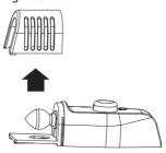
3 Unscrew and remove the old light bulb.
