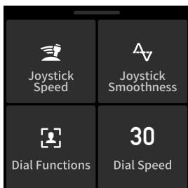
**Joystick Speed:** allows users to control the speed of the joystick for the gimbal. Users can select from fast, medium, slow, and custom. Tap the icon on the top-right of the touchscreen to customize the speed. The larger the value, the faster the joystick speed.
