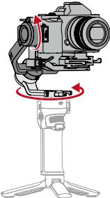
PTF: pan and tilt follow, where both the pan and tilt axes follow the movement of the grip. Suitable for scenarios when moving up and down or on a slant.
