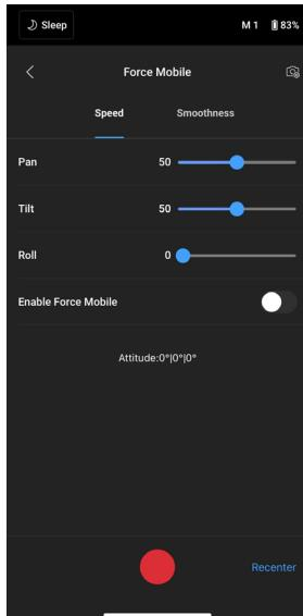
Force Mobile requires the phone holder and a mobile phone mounted on a tripod or handlebar vertically. After enabling this feature in the Ronin app, the gimbal movement can be controlled by tilting and rotating your mobile phone. (The gimbal movement cannot be controlled by rolling the mobile phone by default.)
