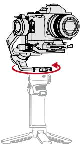
PF: pan follow, where only the pan axis follows the movement of the grip. Suitable for scenarios such as shooting emerging walk-through and arc shots or moving from left to right.
