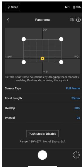
Panorama allows users to capture a series of interconnecting still images with precise control based on the sensor type, lens focal length, overlap, and interval.
