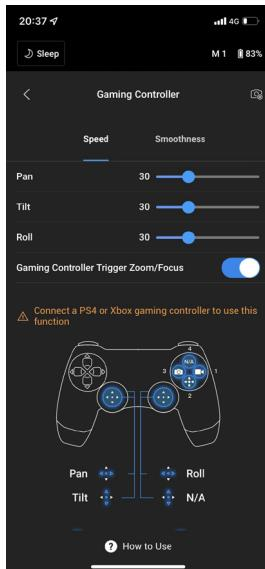
PS4 DualShock and Xbox controllers can be used to control the gimbal and camera. After connecting the controller to the mobile device and gimbal, users can control gimbal movements, focus, and zoom, and can record videos, recenter gimbal, switch user profile, and capture images.
