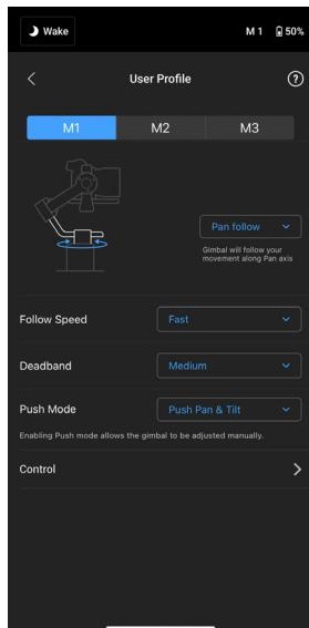
On this page, users can customize parameters in different user profiles such as Follow Speed, Deadband, and Push Mode.
