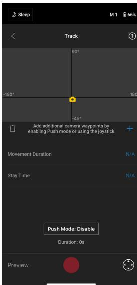
Track is designed to capture video with up to 10 waypoints. Users need to select the waypoint manually by moving the gimbal or using the virtual joystick. The duration parameter below the grid map indicates how much time it will take for the gimbal to travel from one waypoint to the next. The stay time indicates how long the gimbal will remain steady at the waypoint before moving to the next waypoint.
