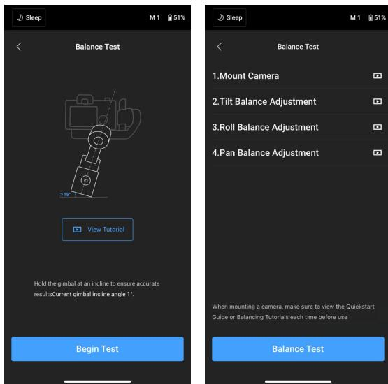
Tap Begin Test to check the balance status and provide a score for each axis. If the balance status is not good, view the on-screen tutorial videos on how to balance. Ensure the gimbal is held at an incline between 15° to 45° before starting the test.
