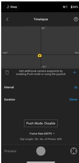
In Timelapse, DJI RS 3 Mini triggers the camera to capture still images with a set interval time and will automatically stop when completed. The duration for the Timelapse and the frame rate can be set so that DJI RS 3 Mini can calculate the exact number of images required.
