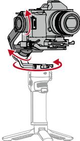
FPV: pan, tilt, and roll follow, where all three axes follow the movement of the grip. Suitable for scenarios when rotating the camera or shooting from a low angle.
