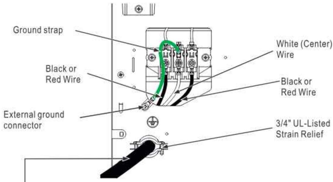
3-10 AWG minimum copper conductors or 120/240 V 30A power supply cord kit marked for use with dryers and provided with closed loop or spade terminals with upturned ends(not supplied).
