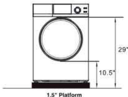
Use 1.5" height platform to make the machine ADA compliant.
