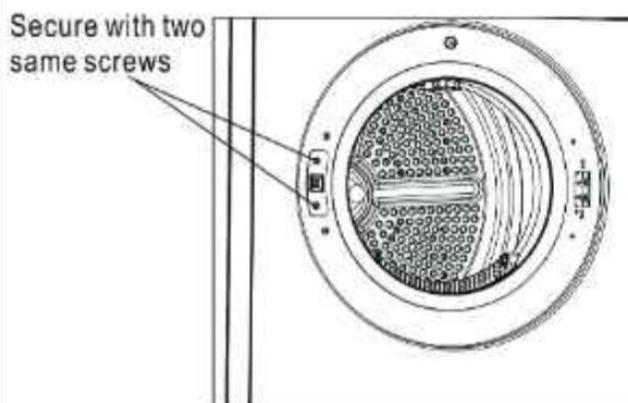
**Step 4.** Rotate and replace the hinge/door assembly on the opposite side, secure them using the same screws.
