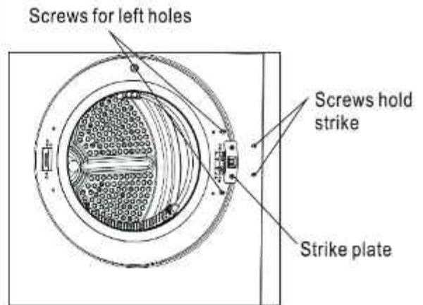
**Step 3.** Rotate the strike plate, then re-install it on the opposite side. And screw the other two screws into the holes left after remove the hinge/door assembly.
