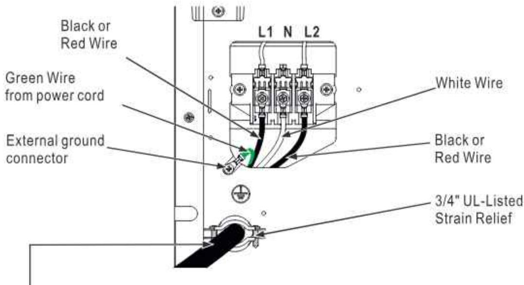
4-10 AWG minimum copper conductors or 120/240 V 30A power supply cord kit marked for use with dryers and provided with closed loop or spade terminals with upturned ends(not supplied).
