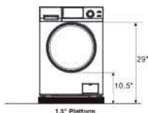
Use 1.5" height platform to make the machine ADA compliant.
