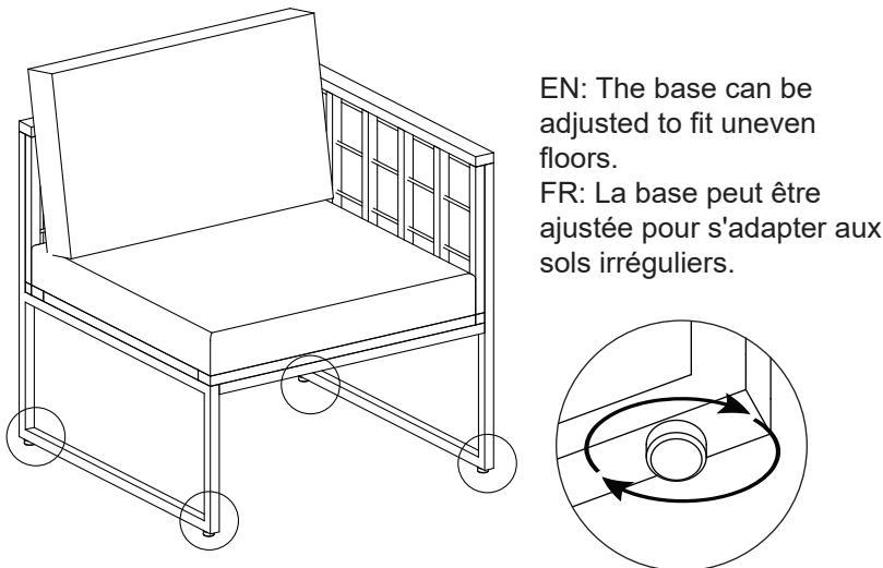
EN: The base can be adjusted to fit uneven floors.
