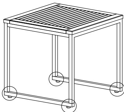
EN: The base can be adjusted to fit uneven floors.
