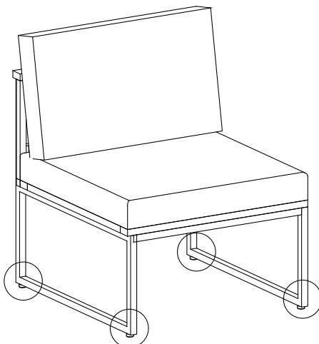
EN: The base can be adjusted to fit uneven floors.
