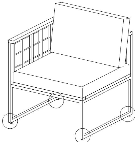
EN: The base can be adjusted to fit uneven floors.
