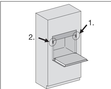
It is a good idea to remove the door (see "Cleaning and care – Removing the door") and the accessories before installing the oven. The oven is then easier to push into the housing unit and you do not run the risk of lifting it by the door handle.
