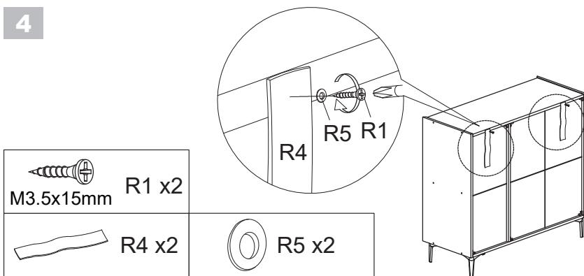
Add safety strap (R4), washer (R5) using 3.5x15mm screw (R1) to back of cabinet.
