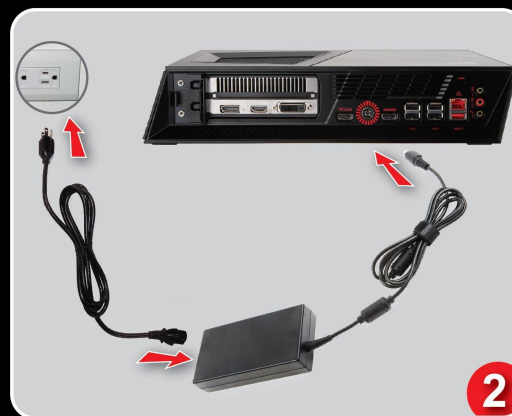
2. Connect the power cord to the system and electrical outlet.
