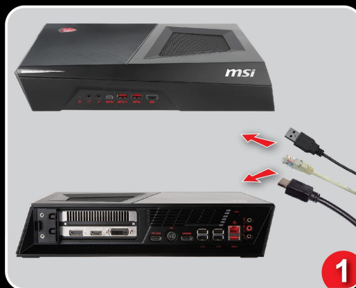
1. Connect the cables of keyboard, mouse, LAN, monitor, etc.
