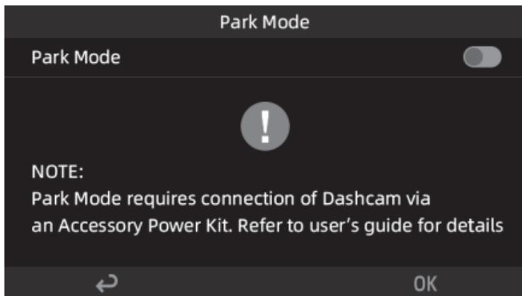
If the G-sensor is triggered, your dash cam wakes up and records one minute of emergency video, then returns to sleep mode. Within one minute, your dash cam checks the G-sensor. If the G-sensor is triggered again, your dash cam starts loop recording for five minutes, then it turns off and enters park mode.
