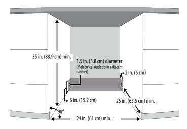
If you are installing the unit between frameless cabinets, a 0.5 in. (1.3 cm) wide filler strip or side panel may be needed on both sides of your cooler. The filler strip provides a space between the appliance case and the adjacent cabinet door swing. The width of the opening must include the filler panels. The door should extend at least 1 in. (2.6 cm) beyond the surrounding cabinets.
