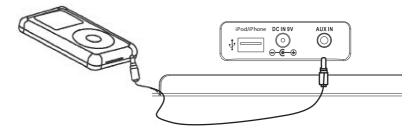
3 Press **SOURCE** repeatedly on the top of your boombox to select **AUX** In. "AUX" lights up on the display.
