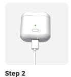
Plug the small end of cable into charging port of charging base.
