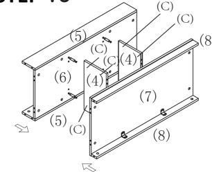
Install 2 Between panels (4) to the middle of Solid panel (6) and Solid panel (7), then lock with 8 pcs Cam locks (C) Part C x 8
