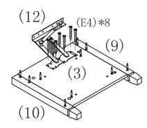
Install lever (12) to End panel (3) with 8 pcs Screws (E4) Part E4 x 8 Part 1 2 x 1
