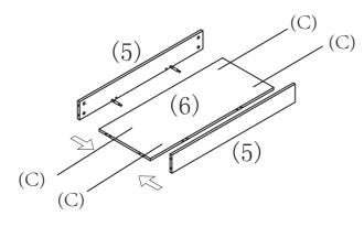
Attach 2 Brace panels (5) to Middle panel (6) and lock with 4 pcs Cam locks (C) Part C x 4  $\,$
