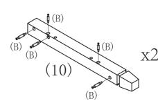
Install 8 pcs cam pins (B) to 2 Legs (10) Part B x 10 Part 10 x 2
