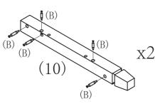
Install one Front Leg (9) and one Rear Leg (10) to End panel (2) and lock with 4 pcs Cam locks (C) Part C x 4
