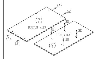
Install 4 pcs dowels (A) and 4 pcs cam pins (B) to Bottom panel (7) Part B x 4 Part 7 x 1 Part A x 4
