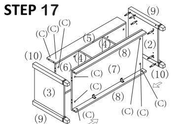
Integrate End panel (2), (3) and the table legs with the main body, then secure with 20 pcs Cam locks (C)
