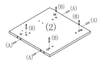
Install 4 pcs dowels (A) and 4 pcs cam pins (B) to End panel (2) Part A x 4 Part B x 4 Part 2 x 1
