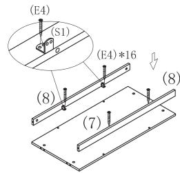
Install 2 Support panels (8) to Bottom panel (7) with 16 pcs Screws (E4) and reinforce with 4 sets of Corner brackets (S1) (S1 has equipped with self-tapping screws with no drilling holes)
