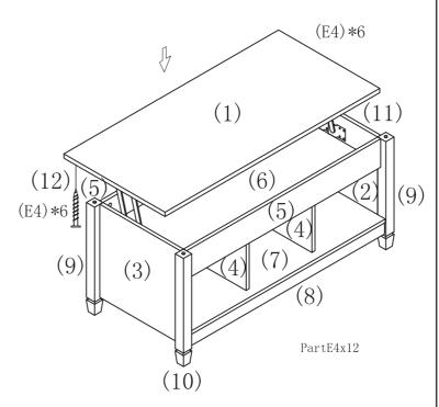
Install the Top panel (1) to the lifters (11), (12) with 12 pcs Screws (E4)
