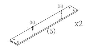
Install 4 pcs cam pins (B) to 2 Brace panels (5) Part B x 4 Part 5 x 2
