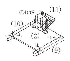
Install lever (11) to End panel (2) with 8 pcs Screws (E4) Part E4 x 8 Part 11 x 1
