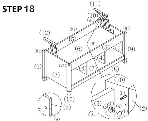
Stick 40 pcs Cam covers (P) on Cam locks (C) and stick 6 pcs (M1) to the corresponding places shown in the figure.
