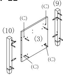
Install one Front Leg (9) and one Rear Leg (10) to End panel (3) and lock with 4 pcs Cam locks (C) Part C x 4
