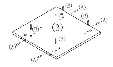
Install 4 pcs dowels (A) and 4 pcs cam pins (B) to End panel (3) Part A x 4 Part B x 4 Part 3 x 1
