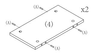
Install 8 pcs dowels (A) to Between panel (4) Part A x 8 Part 4 x 2
