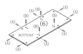
Install 8 pcs dowels (A) and 4 pcs cam pins (B) to Middle panel (6) Part B x 4 Part A x 8 Part 6 x 1
