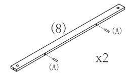
Install 4 pcs dowels (A) to 2 Solid Panels (8) Part A x 4 Part 8 x 2
