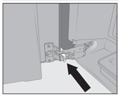
■ Remove the door opening limiters from the hinges, e.g., by prizing them out with a screwdriver.
