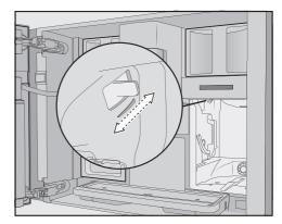
Push the slide control exactly 1 setting forward (for finer grinding) or one setting backward (for coarser grinding).
