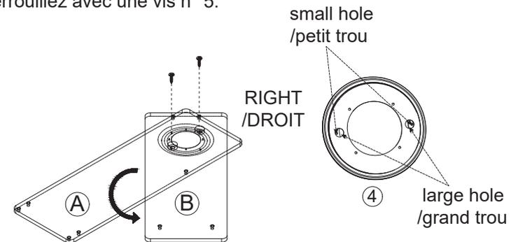
Rotate Part B so that the two large holes on Part B align with the two small holes on Part A.
