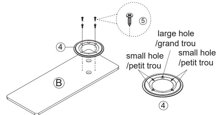
Align Part B with the right side of Part A, rotate Part B, align the large hole of Part B with the small hole of Part 4, and align the small hole of Part 4 with the small hole of Part A, and lock it with the No. 5 screw.
