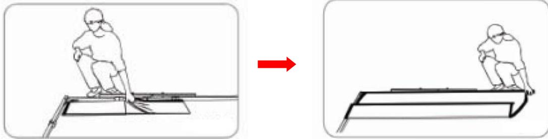
2. Once the screen material is fully extended, secure the material by snapping the buttons onto the frame studs. Fasten the buttons in the following order as shown on **Fig.1**.
