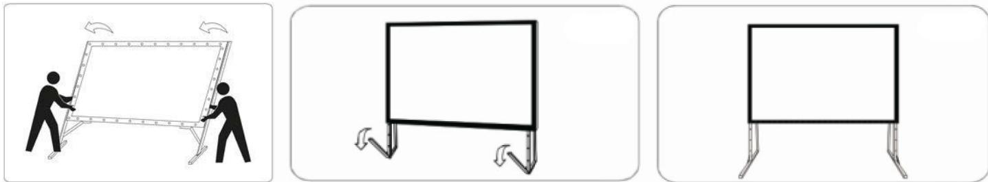
4. The assembly is now complete, and the projection screen will be stable on a flat surface.
