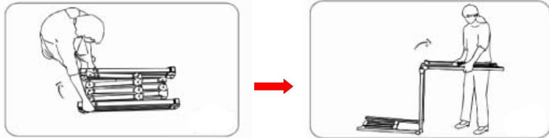
2. Next, unfold the frame until the latch on the hinge “clicks” into place. Repeat the procedure for the shorter sections, as shown below.
