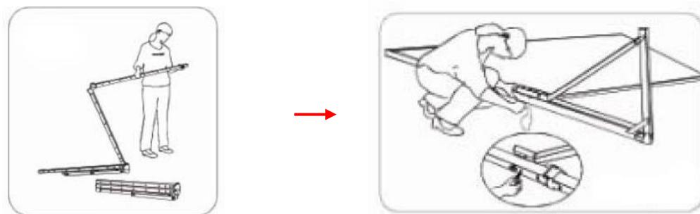
3. After making sure the legs are secure to the frame, using two people, lift the screen up in a vertical position. While the screen is in a vertical position, fold the front feet of the legs out.
