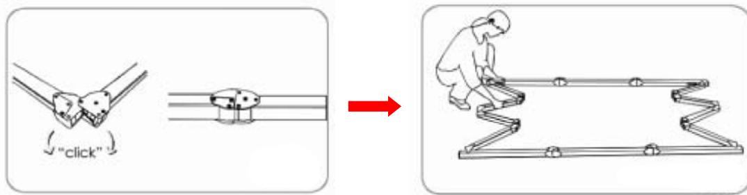
**Note:** When unfolding the frame and legs, be sure the latches on the hinges "click" into place. Please also make sure all 4 corners of the frame are at a 90° angle and the hinged support bar is straight and not bent.
