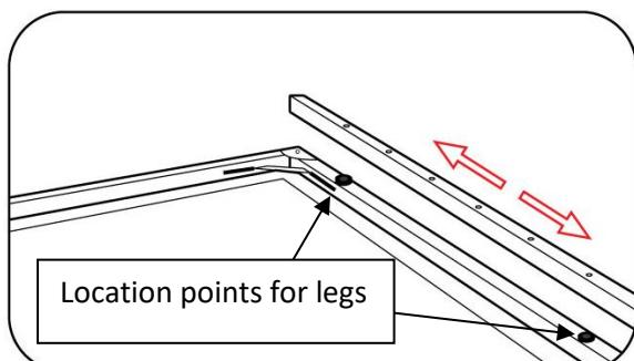
Step 2: Once you have aligned the leg's holes with the frame's holes, secure with the knob screws.
