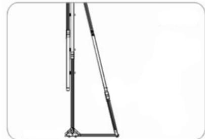
2. Next, carefully unfold the extra support leg behind the leg and attach it securely using a **knob screw (C)**. Then repeat steps 3 and 4 on the previous procedure.
