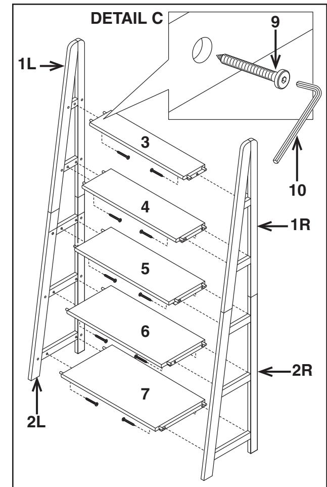
**Remove all parts from carton, separate by part numbers indicated on parts list, and verify part quantities.**
