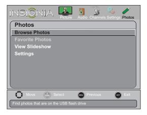
4 Press ▲ or ▼ to highlight Browse Photos, then press ENTER. The screen displays folder names and photo files stored on the USB flash drive in a thumbnail index with the first photo or folder highlighted. A control bar appears at the bottom of the screen.
