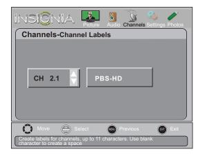
4 Press ▲ or ▼ to select the channel you want to label, then press ► to move to the channel label field.
