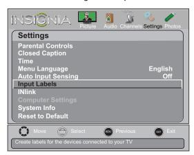
3 Press ▲ or ▼ to highlight Input Labels, then press ENTER. The Settings-Input Labels screen opens with the input source field highlighted.
