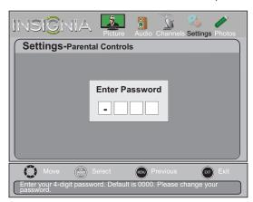
**4** Press the number buttons to enter the four-digit password. The *Settings-Parental Controls* menu opens.
