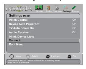
4 Press ▲ or ▼ to highlight Connect, then press ENTER. A HDMI CEC-compatible device in standby mode turns on.
