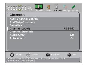
3 Press ▲ or ▼ to highlight Channel Labels, then press ENTER. The Channels-Channel Labels screen opens with the channel number field highlighted.
