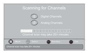
During scanning, your TV searches for digital channels first. When the digital channel search is complete, a message appears asking if you want to search for analog channels. Select **Yes** to continue searching for analog channels, or select **No** to stop searching for channels.
