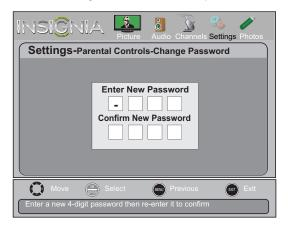
**6** Press the number buttons to enter a password, then enter the password again. "Password successfully changed" is displayed.
