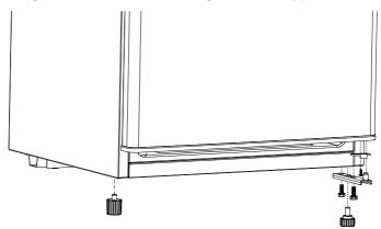
7 Install the leveling foot you removed from the left side into the right bottom of your refrigerator.
