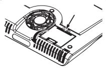
2 Pull the USB cable from inside the compartment, then clip the cable into the cable guide.
