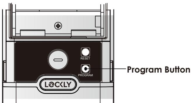
To enter **Programming Mode**, remove the battery compartment cover on the interior side of the Secure to expose the **Reset** and **Program** buttons.
