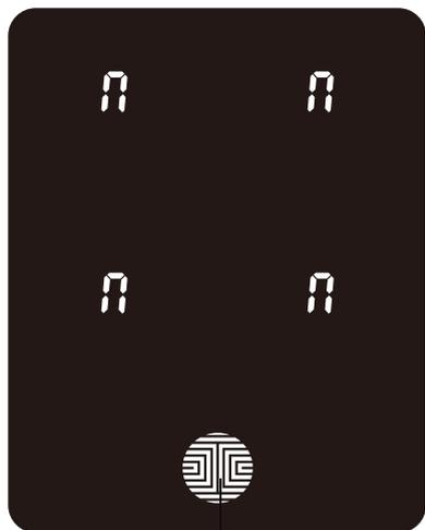
If the two (2) **Access Codes** you entered does not match, an error message will appear on the screen (As shown to the left). Press **OK** to return to the **Programming Screen** and try again. See **Section 3.3**
