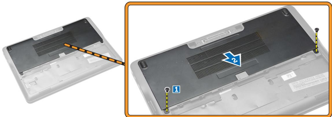
4. Lift the base cover to remove it from the computer.
