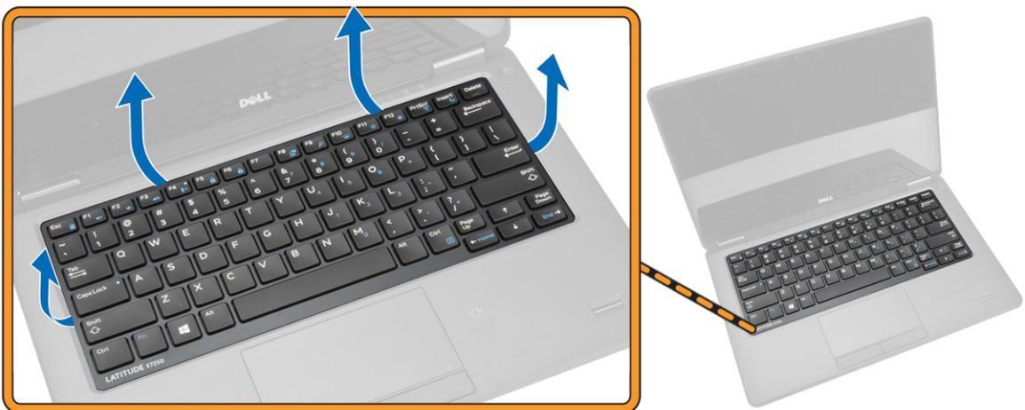
4. Lift up to remove the keyboard trim from the computer.
