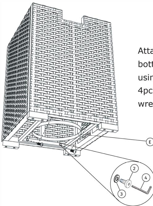
Attach metal stand (E) to bottom of gas tank cover using 4pcs of Bolts (2) and 4pcs M6 washer (3) with Allen wrench (4). Fully tighten.
