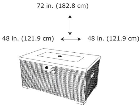
Combustible materials should not be within 60 inches of the top of the unit, or within 48 inches around the entire unit.
