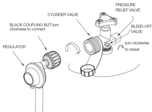
Before performing a leak test, be sure that no sparks can occur and you are in a spacious outdoor area. Connect the propane gas tank to the regulator and turn the valve on the unit to the "off" position. Brush a soap and water mixture on all connections. Turn the gas supply on; if bubbles occur on any connection there may be a leak. If you smell gas or a leak is discovered turn the gas valve off, disconnect propane gas tank and do not use the appliance until the leak is repaired.
