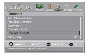
3 Press ▲ or ▼ to highlight **Channel Strength**, then press **ENTER**. The signal strength meter is displayed.
