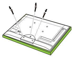
**4** Attach the wall-mount bracket to your TV using the mounting holes on the back of your TV. See the instructions that came with the wall-mount bracket for information about how to correctly hang your TV.
