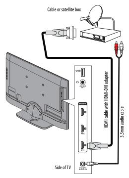
5 Connect a 3.5mm audio cable (not provided) to the PC/DVI AUDIO IN jack on the side of your TV and to the AUDIO OUT jacks on the cable or satellite box.
