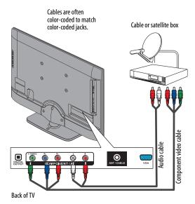
4 Connect an audio cable (not provided) to the L and R audio jacks on the back of your TV and to the audio out jacks on the cable or satellite TV box.
