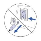
Turn the printer off, remove the power cord and AC adapter, and open the cover.
