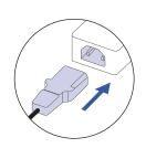
Connect the power cord to the AC adapter.
