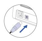
First, connect the AC adapter jack to the printer
