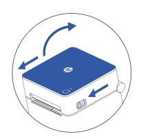
Press on both release levers on the sides of the printer to unlock the printer cover.
