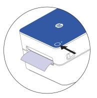
Once printer cover is closed label should align on its own. If it doesn't, press the feed button to align the label.
