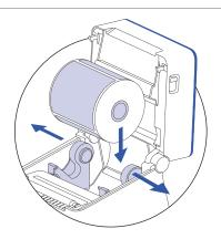
Lift the printer cover and insert a roll of labels between the media holders.
