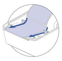
Feed the end of the label roll under the two media holder guides in the printer before placing the end of the roll on the printing slot. Then, close the printer cover.
