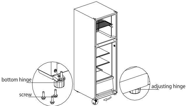
5 Dismantle the limit blocks and screws on the lower cover of both refrigerator door and freezer door, install them on the other side of both doors; then install the sleeve pipe on the upper cover of the refrigerator door on the other side.
