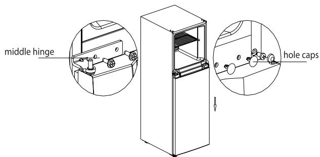
7 Install the freezer door on the middle hinge, and install the upper hinge, hinge cover and hole cover.
