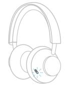
Once successfully connected, AirFly Pro will illuminate in white and remain on for 10 seconds.
