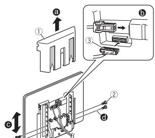
**4 Secure the monitor cables to the hook on the back of the LCD screen then attach the monitor cover (①) by using the screws (②).**
