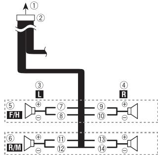
Perform these connections when using a subwoofer without the optional amplifier.
