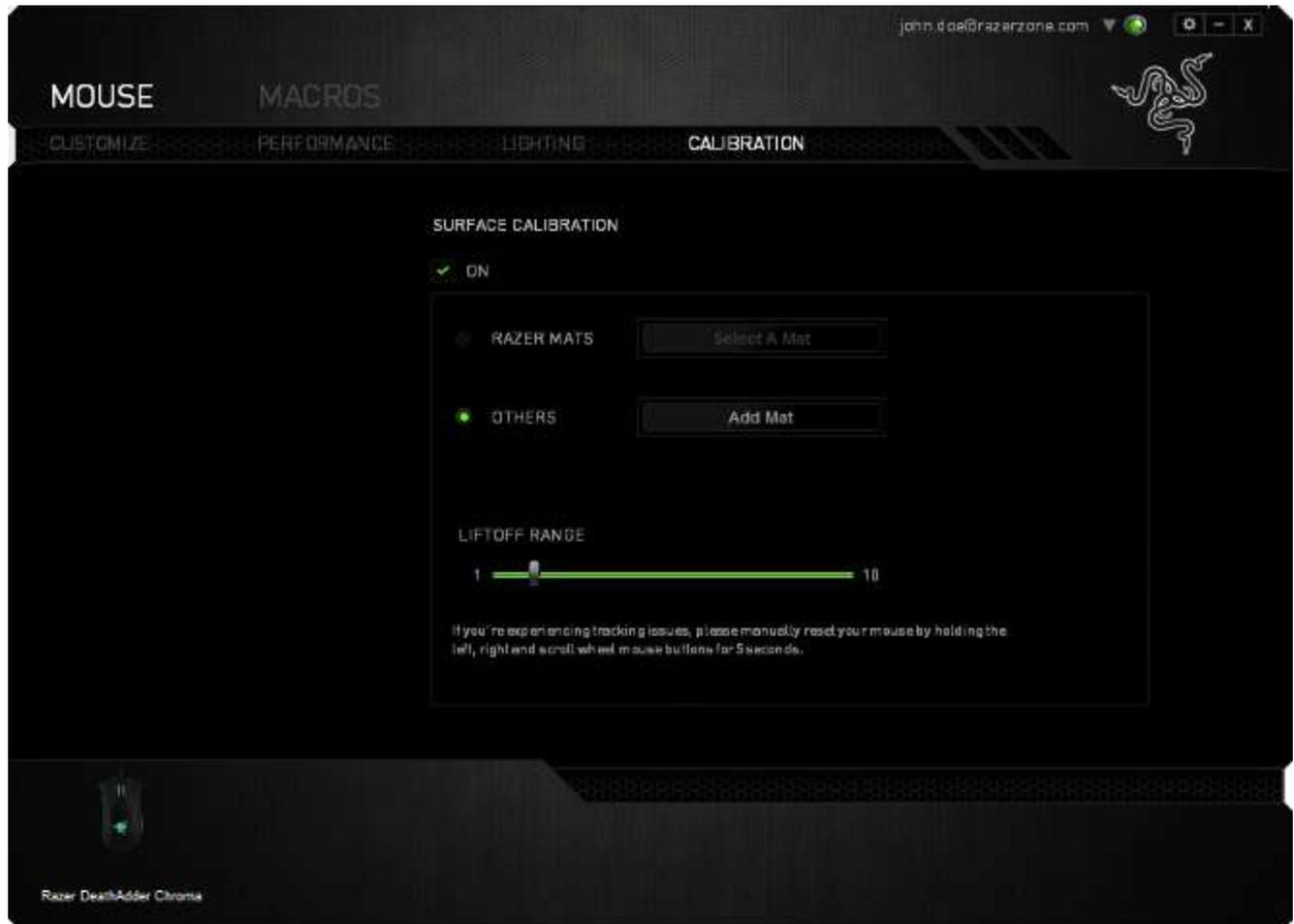
This submenu enables you to manually adjust the Razer Precision Sensor to suit any mousing surface.
