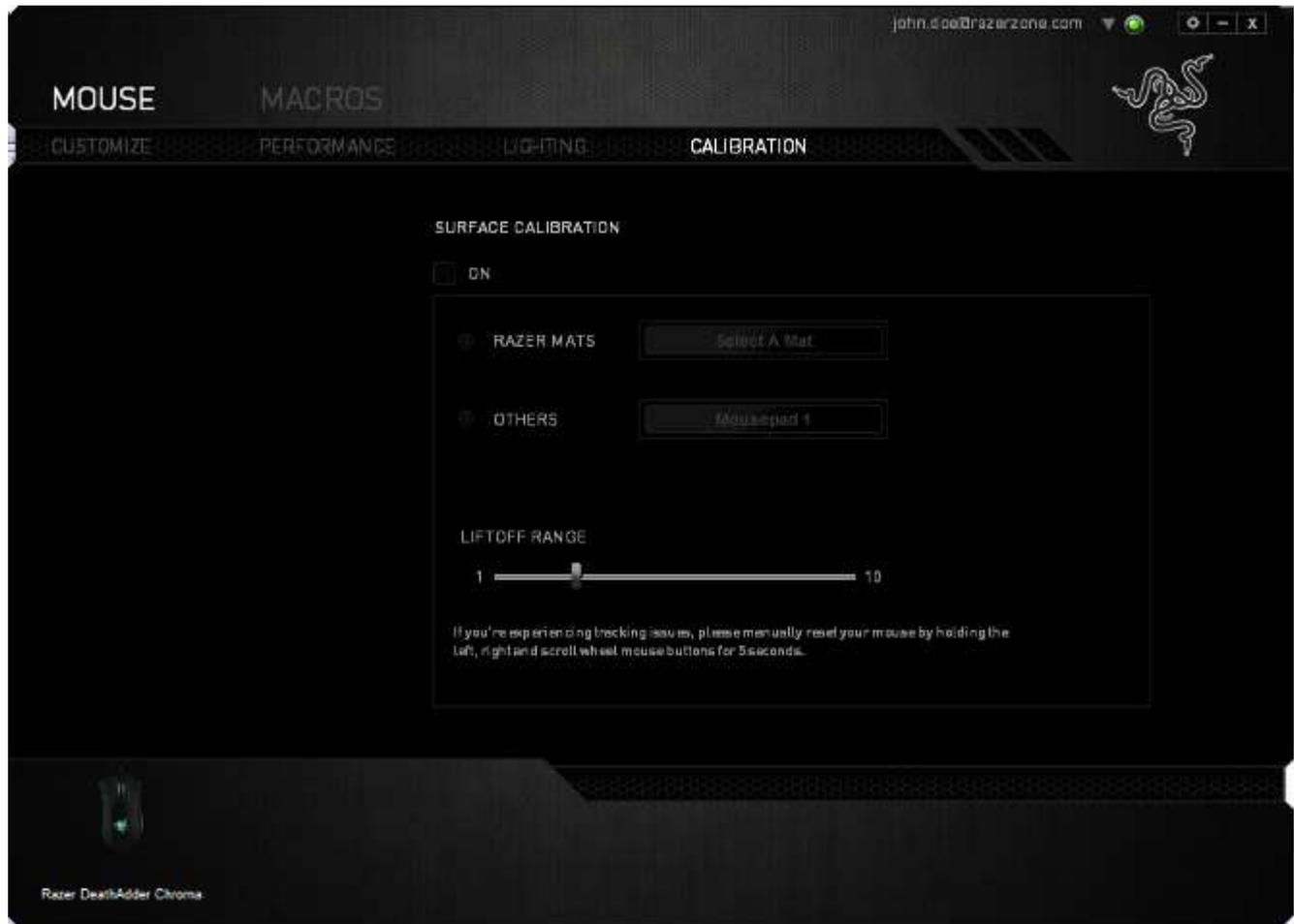
The *LIFTOFF RANGE* allows you to set the distance in which the sensor stops tracking as it is being lifted away from its mousing surface. To use this feature, you must first activate *SURFACE CALIBRATION* then choose an appropriate mousing surface.
