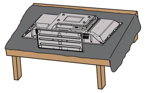
2 If the stand is attached, remove the three screws that secure the stand column to the TV, then remove the stand column.
