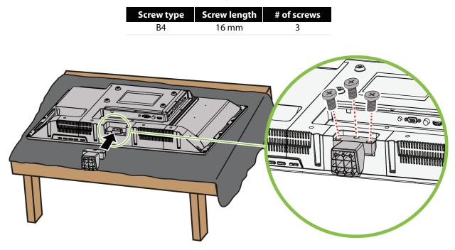
3 Secure the TV stand the TV with the four provided  $B4 \times 18$  mm screws (these are the long screws).
