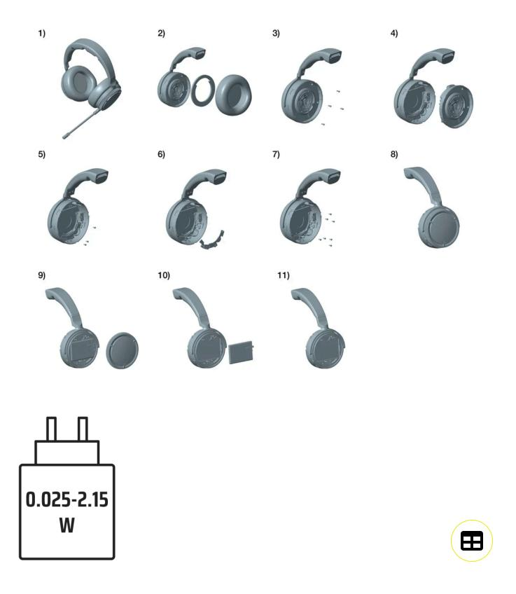
The power delivered by the charger must be between min 0.025 Watts required by the radio equipment, and max 2.15 Watts in order to achieve the maximum charging speed.
