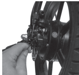
Pinch and tighten the brake cable
