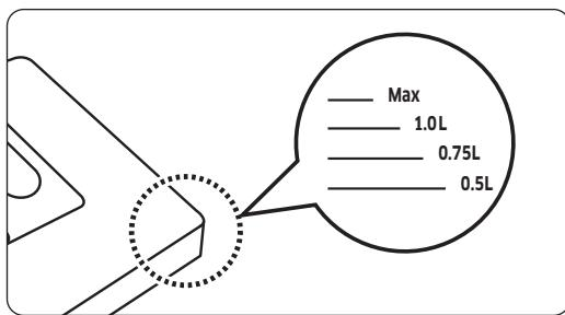
2. Open the reservoir cap and then fill the reservoir with tap water.
