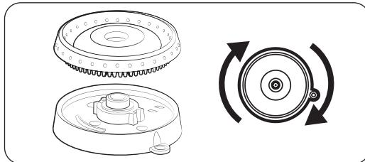
1. Put the burner heads on the burner bases as shown at left. (The bottom of the head fits inside the top of the base.)
