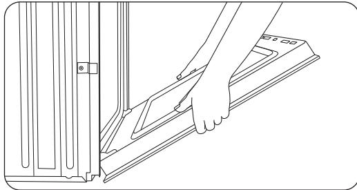
9. Holding the door at a 45° angle, insert the hinges in the slots. (A slight drop engages the hinges.)
