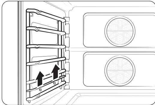
1. Grasp the bottom-center of the support and lift.
