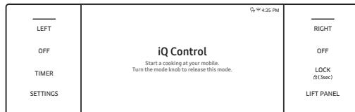
Tap **SETTINGS > Connections > iQ Control > ON** (for the appropriate oven).
