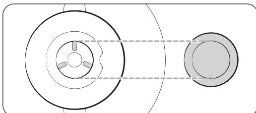
1. Orient the burner head so the electrode opening aligns with the electrode.
