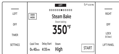
4. The new steam level appears on the main screen. Important: Fill the water reservoir before cooking. (See **Using the Water reservoir**, Pg. 9)
