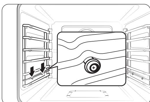
6. Pull the rack support down, making sure the two humps on the support bar rest upon the nuts attached to the oven-chamber wall.
