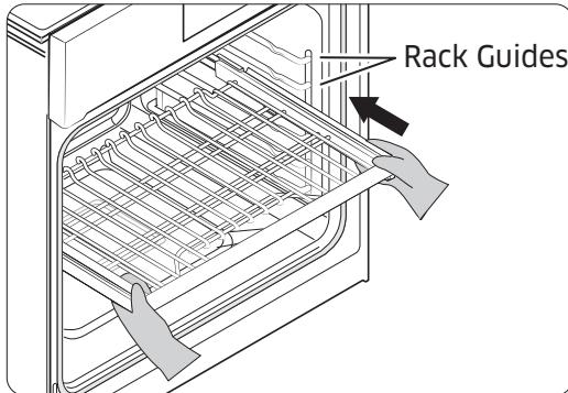
With the gliding rack slides retracted and the oven off, insert the rack between the guides until the rack reaches the back.
