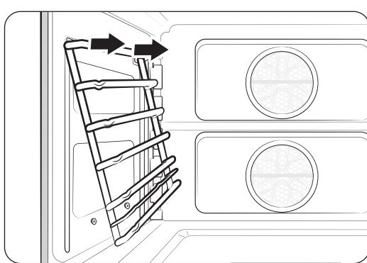
3. Pull the rack support from the mounting holes.
