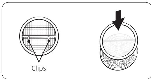
Centering the filter over the fan hole, carefully hook the metal clips (back of filter) over the metal bar across the hole. Do not scratch the oven's porcelain with the filter.
