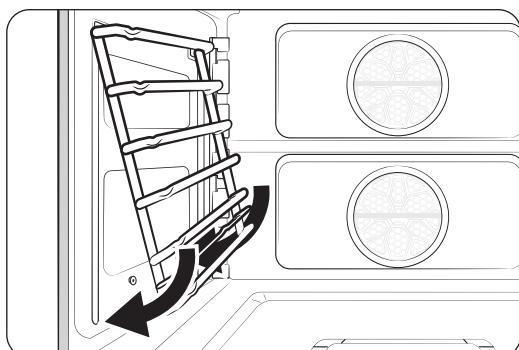
5. Swing the bottom of the rack support toward the oven-chamber wall.
