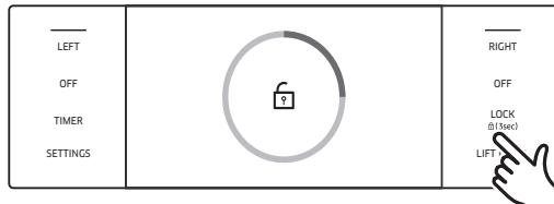
Touch-hold **LOCK** for 3 seconds. The control lock confirmation and lock icon disappear.
