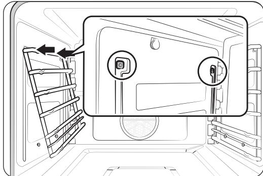
4. Insert the rack-support prongs into the holes near the top of the oven-chamber wall.
