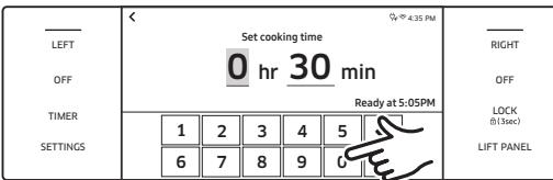
3. Tap numbers on the numeric pad to set the cooking time (from 1 min to 9 hrs 59 min's).
