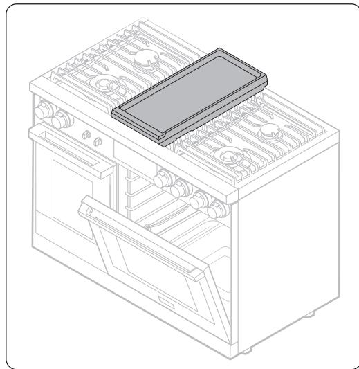
1. With all burners off and the range cool to the touch, place the griddle and grate in the center of range.
