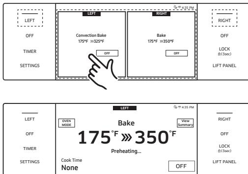
If using the ovens in single mode, tap the **LEFT** or **RIGHT** area on screen, then tap the temperature area and use the number pad to enter a new temp.
