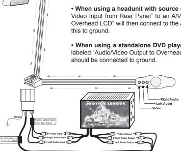
**Note:** This cable is intended for use in conjunction with an RP5-GM32 to retain all safety and convenience systems. The vehicle should be equipped with an overhead LCD and IR system, in which the DVD player was part of the AM/FM/CD receiver. The RP5-GM32 is needed to power the IR headphone system.
