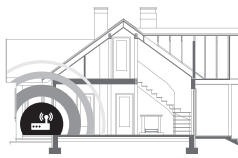
Unsuitable router position
