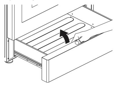
2 To replace the drawer, make sure that the white wheel on the drawer aligns with the rails well, then slide the drawer back into your range.
