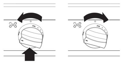
**2** After the burner lights, turn the control knob to the setting you want. The "clicking" sound stops and the flame height changes from Max. to Min. when you turn the control knob.
