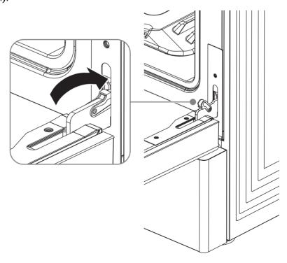
4 Fully close the levers on the left and right hinges, then close the door.
