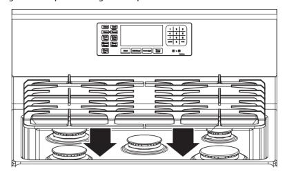
**10** Push in and turn each surface burner control knob to the **LITE** position, let each burner light, then set each control knob back to a burner setting to make sure each burner operates correctly.
