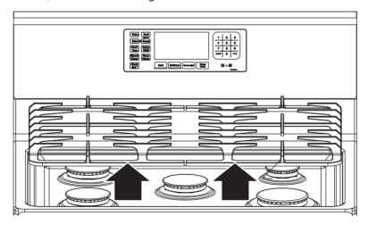
**WARNING:** Do not remove or lift the cooktop during cleaning. Doing so could damage the gas lines leading to the surface burner manifolds, causing poor or dangerous operation.
