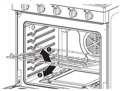
3 Clean by hand in hot, soapy water with a plastic or soap-filled scouring pad, then dry with a soft cloth.
