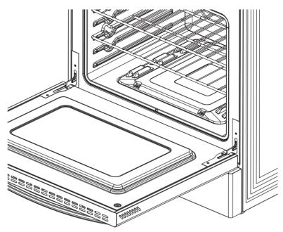
2 Open the levers fully on both sides.
