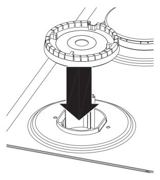
8 Set the burner caps on top of the burner heads. These also need to be flat on top of the burner heads to ensure proper and safe operation.
