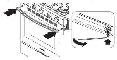
4 Use the Allen wrench to tighten both sides of the door handle.
