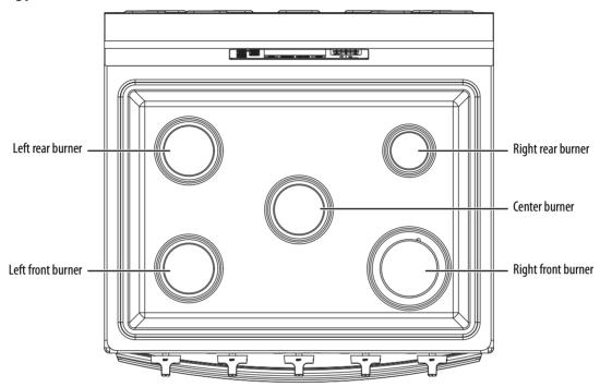
The **right rear** burner provides precise cooking performance for delicate foods and foods that require low heat for long cooking times. The right rear burner lets you use the LO setting for a low simmer setting.
