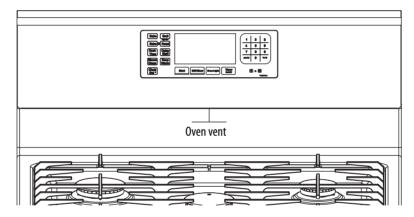
Do not block or place items in front of the oven vent. Correct air circulation prevents oven burner combustion problems and provides good cooking results.
