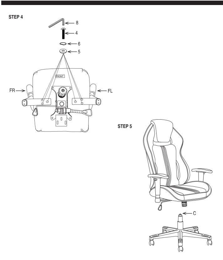
STEP 4 Attach Arms (FL & FR) to Seat Cushion (H) using three Flat Washers (5), three Spring Washers (6) and three Bolts (4) for each arm. FULLY TIGHTEN ALL BOLTS USING ALLEN WRENCH (8).
