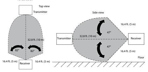
**Note:** The transmitter and receiver must be located within the same room. The wireless signal will not pass through walls, floors, or ceilings.
