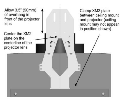
**projector for maximum security**. Alternatively, secure the XM2 plate to a shelf underneath the projector leaving the same extension in front of the projector lens.
