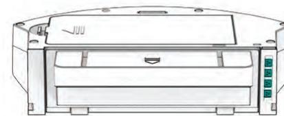
4. Wipe the top and the area around the SLAM LiDAR.
