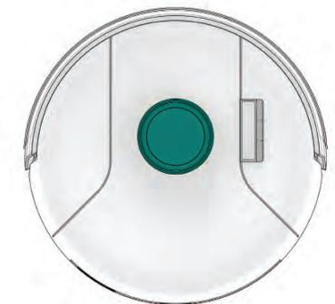
**Important Note:** Austin's SLAM LiDAR is a sensitive sensor. Do not apply force, insert objects, or adjust the SLAM LiDAR. Do not sit or place items on top of Austin.
