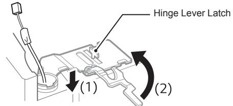
3 Connect the wire harness (1). On the InstaView model, screw in the ground wire.
