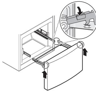
5 Replace the ice bin in the drawer. Insert the Durabase basket in the rail assembly.
