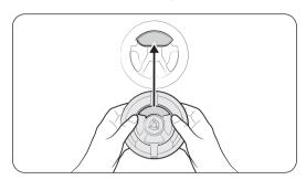
1. Orient the burner head so the electrode opening aligns with the electrode.
