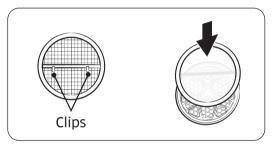
Centering the filter over the fan hole, carefully hook the metal clips (back of filter) over the metal bar across the hole. Do not scratch the oven's porcelain with the filter.
