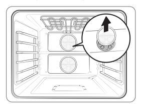
When the oven is cool, grasp the edges of the filter, and gently push up.
