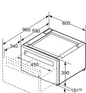
measurements in mm
