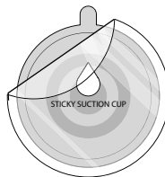
1. Peel off the protective film on the Suction Cup and press firmly onto the windshield.
